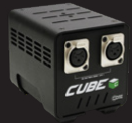
CUBE-200 Input Voltage: AC 100-240V 50/60Hz DC Output: 200W max(14.3v) via 4pin XLR Protection: Over Current, & Temperature Dimensions: 4.8" x 3.3" x 3.7" Weight: 1.4lbs.
